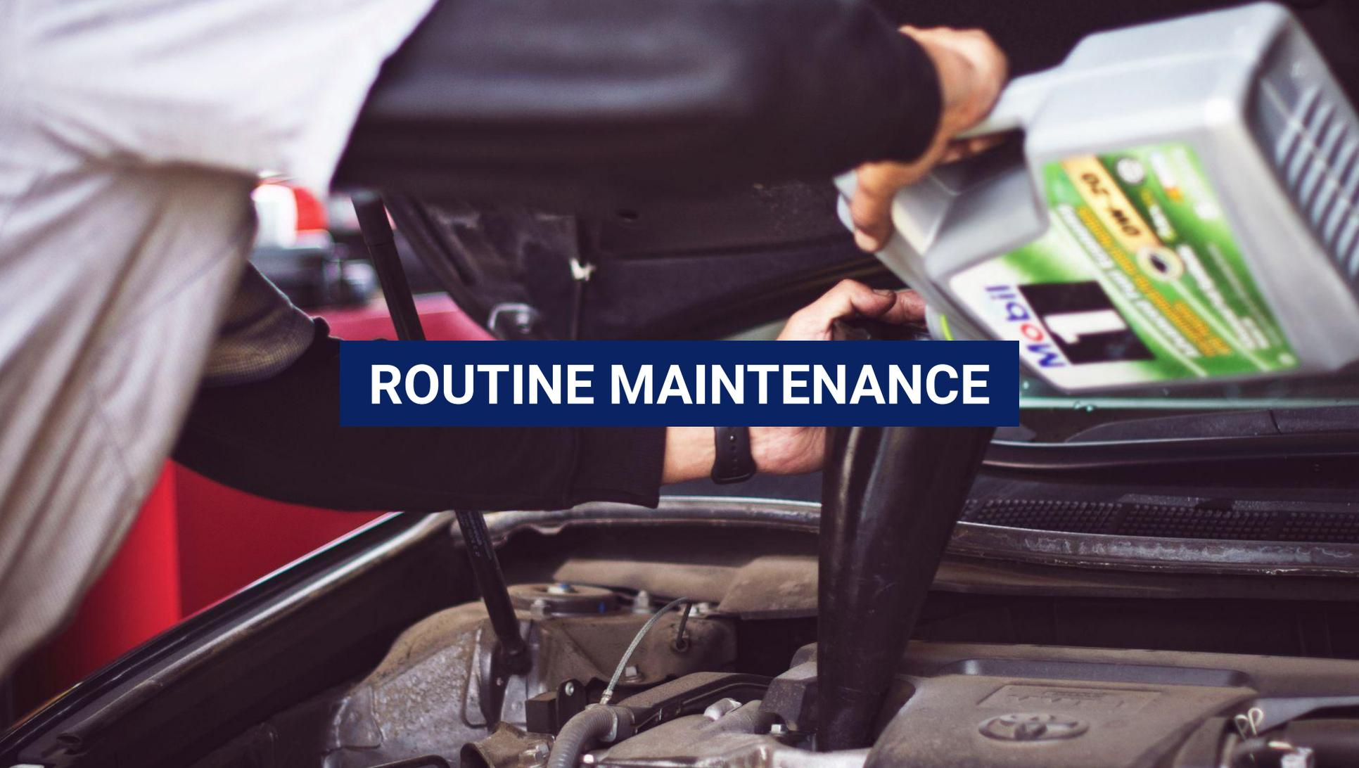
A close-up photograph of a mechanic in a black uniform pouring oil from a grey and green Mobil 1 5W-20 oil jug into a car's engine. The mechanic's hands are visible, one holding the jug and the other near the engine. The engine bay is open, showing various components like hoses and the oil filler neck. The background is slightly blurred, showing a red car and a white wall. A dark blue banner with white text is overlaid across the middle of the image.
